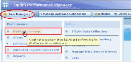
OMEGAMON XE for DB2 PE on z/OS reuses the Optim Performance Manager Extended Insight monitoring capability.. Health Summary and Extended Insight Dashboard are enabled for monitoring of SQL access DB2 for z/OS.
